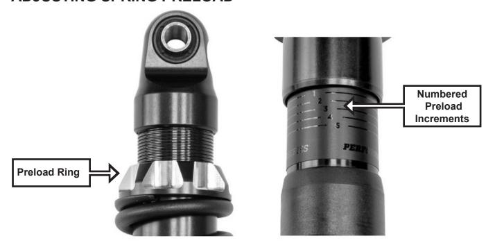
FOX Street Performance RC1 and Street Performance IFP shocks are equipped with spring preload adjusters.
