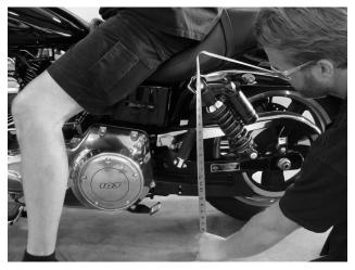
Use a motorcycle floor jack when installing shock absorbers to remove the load on mounting hardware. Torque all hardware to manufacturers specifications.
