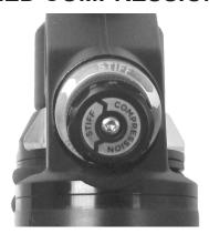
The compression adjust feature on your FOX Street Performance RC1 shocks gives you the ability to externally adjust the shocks compression damping. Adjustments are made by turning the black \ compression knob on the body cap end. The compression damping affects how quickly the rear shock compresses when the motorcycle travels over bumps and depressions on the road.
