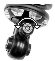
The rebound adjust feature on your FOX Street Performance RC1 shocks gives you the ability to externally adjust the shocks rebound damping. Adjustments are made by turning the black \ rebound knob on the eyelet, located on the end of the shock absorber. The rebound damping affects how quickly the rear shock extends (rebounds) after the motorcycle travels over bumps and depressions on the road.
